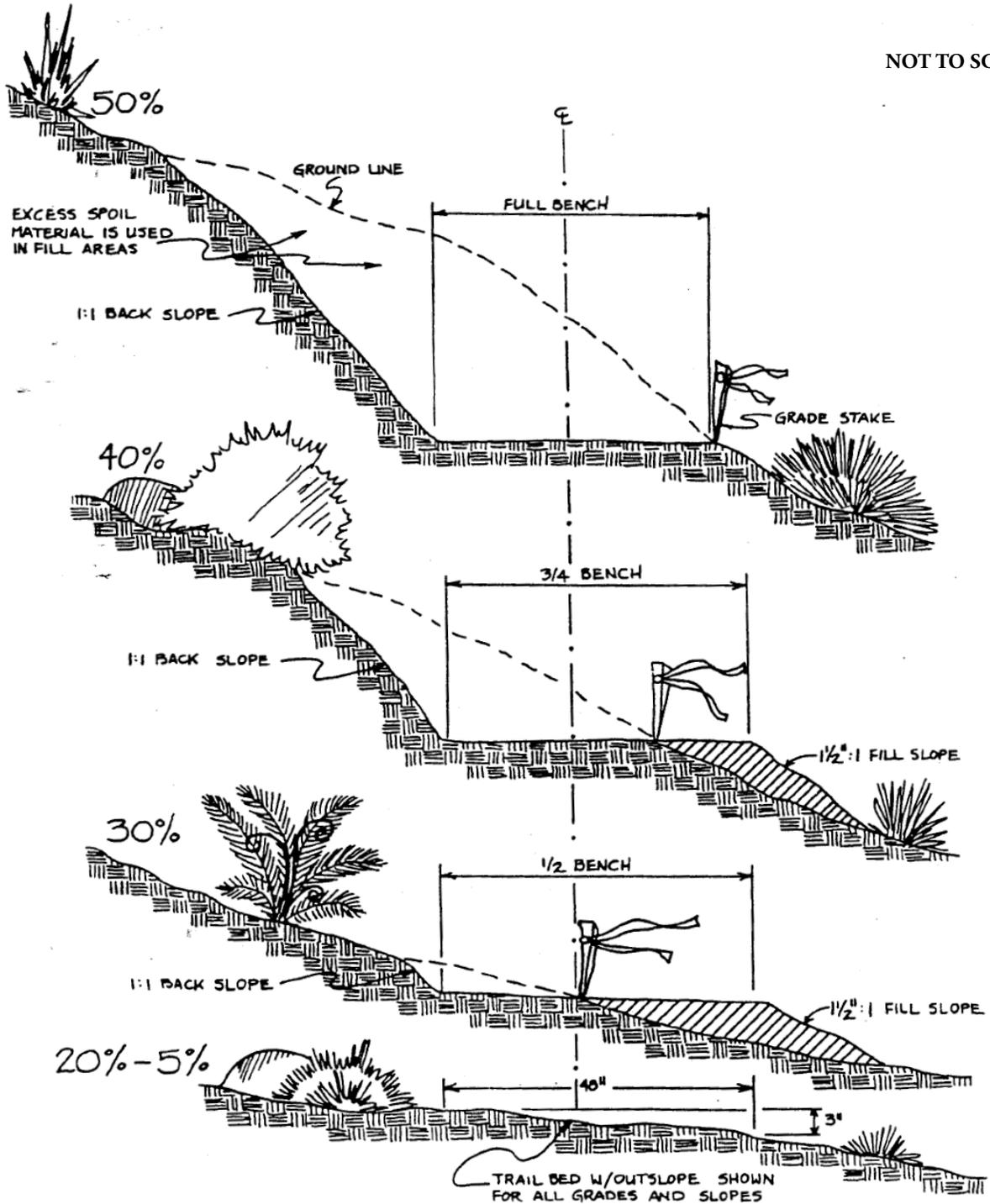
NOTE: AMOUNT OF BENCH VARIES LINEARLY W/% OF SIDE SLOPE. ALL GRADE STAKES INDICATE GRADE AT MINERAL SOIL. ALL FILL TO BE MINERAL SOIL W/NO VEGETATION DEBRIS.
